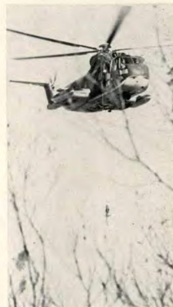
HH-3C rescue helicopter is armor plated, equipped with extensive communications gear and rescue equipment. Injured man on stretcher, left, is assured of rapid trip to medical facility.
